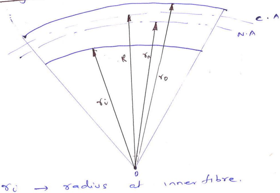
$r_0 \rightarrow$  radius at inner fibre.
