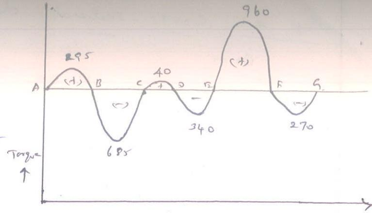
$$\begin{aligned}\text{Energy at D} &= E - 390 + 40 \\&= E - 350\end{aligned}$$
