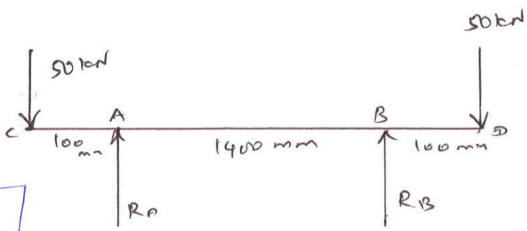
$$\text{Max B.M} = M = 50 \times 10^3 \times 100 \\ = 5 \times 10^6 \text{ N-mm}$$
