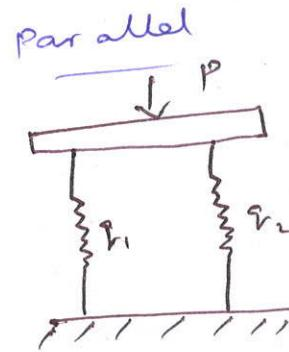
where  $q \rightarrow$  spring rate  $= \frac{P}{y} = \frac{\text{load}}{\text{deflection}}$
