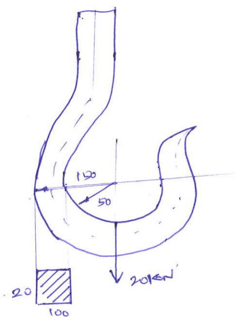
③ A crane hook has a circular C-S as shown in figure. made of plain carbon steel 55C8 ( $\sigma_y = 420 \text{ N/mm}^2$ ). The load acting on the hook is 110 kN. calculate the dimensions of the hook, if the factor of safety as 8.
